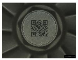
Example automotive components engraved with DMX codes
